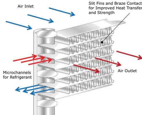
Microchannel coils are all-aluminum coils with fully-brazed construction. This design reduces risk of leaks and provides increased coil rigidity — making them more rugged on the jobsite. Their flat streamlined tubes with small ports and metallurgical tube-to-fin bond allow for exceptional heat transfer.
