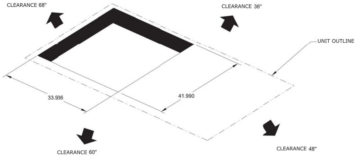
Figure 7. Cooling with optional electric heat models — manual damper — 3-5 tons
