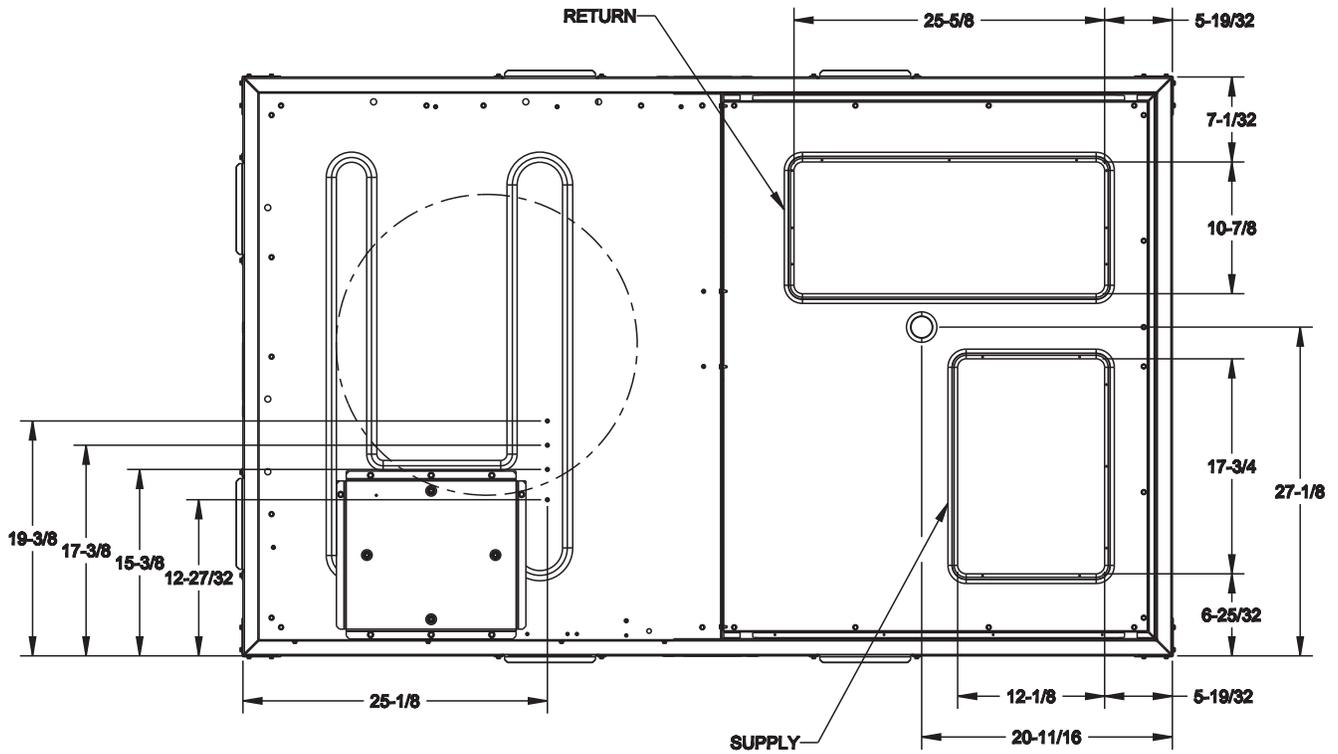
Figure 4. Cooling with optional electrical heat — back view (horizontal configuration) — 3-5 tons
