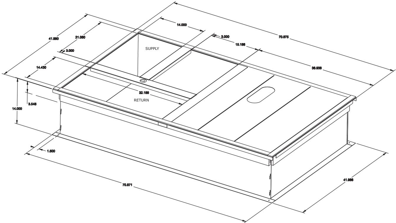
Figure 6. Cooling with optional electric heat — downflow unit clearance — 3-5 tons
